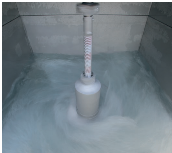
Level-controlled agitator inside the mixing tank at a high and a low filling level: A float guarantees that the agitator is always in the ideal position for mixing, depending on the filling level.
