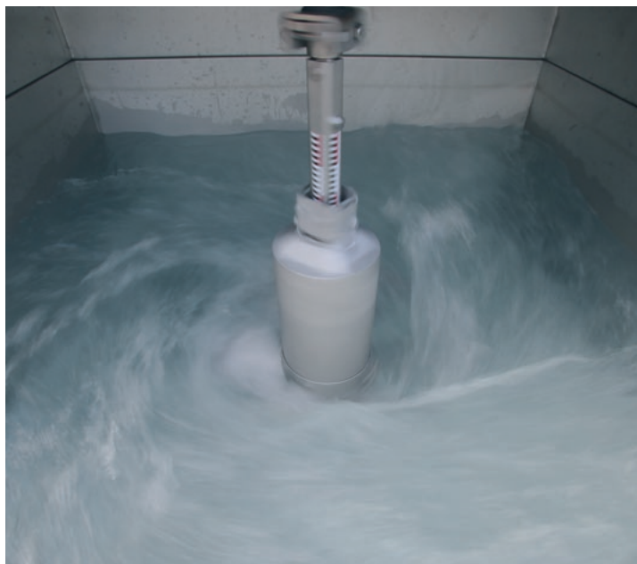
Level-controlled agitator inside the mixing tank at a high and a low filling level: A float guarantees that the agitator is always in the ideal position for mixing, depending on the filling level.
